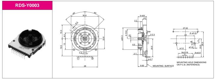
Outer Shaft: Pulse Switch (2Bit Output Signal = 360° Endless (36° step))
